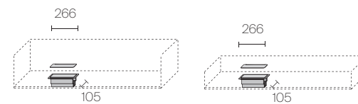
Integrated multiple socket available in European, CH, UK and USA configurations
